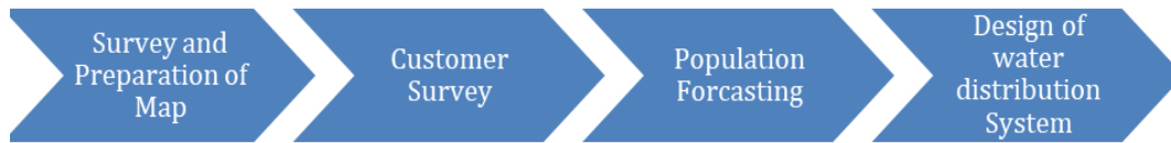
Fig. 1 : Schematic diagram of steps for designing water supply System
