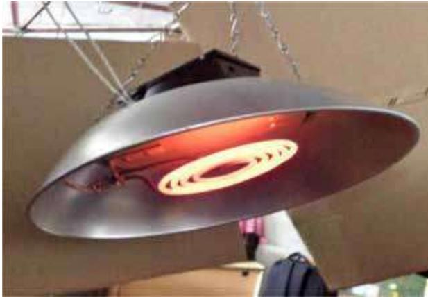
**Fig. 7. Electric Brooder**
