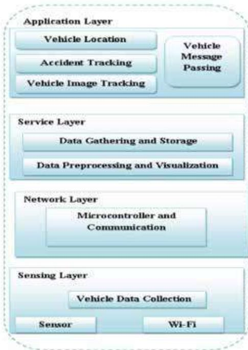
**Fig. 1. Layered design of the planned ATM system**
