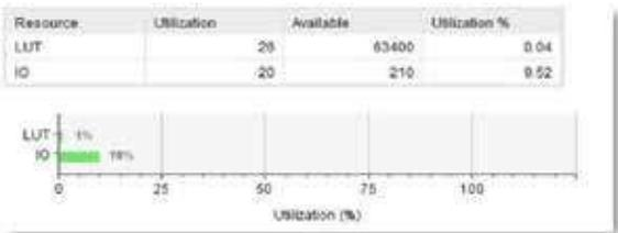
**Fig. 19. Device Utilization Summary of Array Multiplier**
