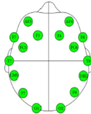
Figure 1: Emotiv EPOC electrodes placement
