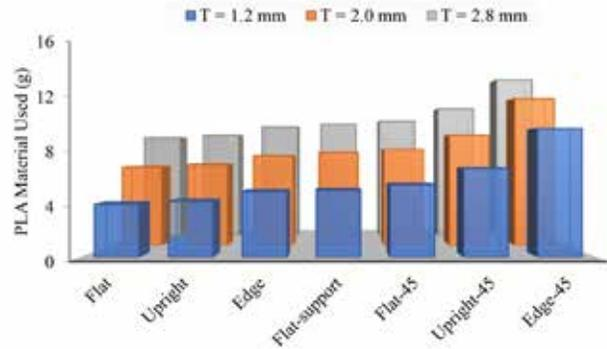
**Figure 5 Amount of PLA filament used for different build orientation**
