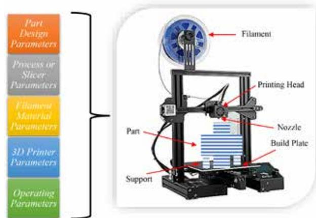
**Figure 1: Typical FDM 3D printing setup and its parameters**
