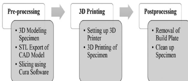
**Figure 3** Three stage 3D printing process
