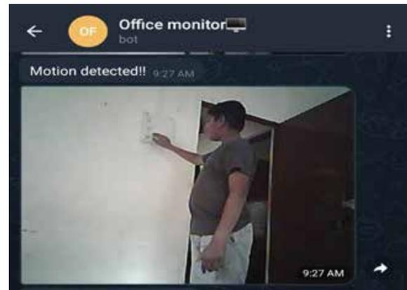
**Fig. 5 Alert message and image of the person interfering is sent to a telegram bot named “Office monitor”.**
