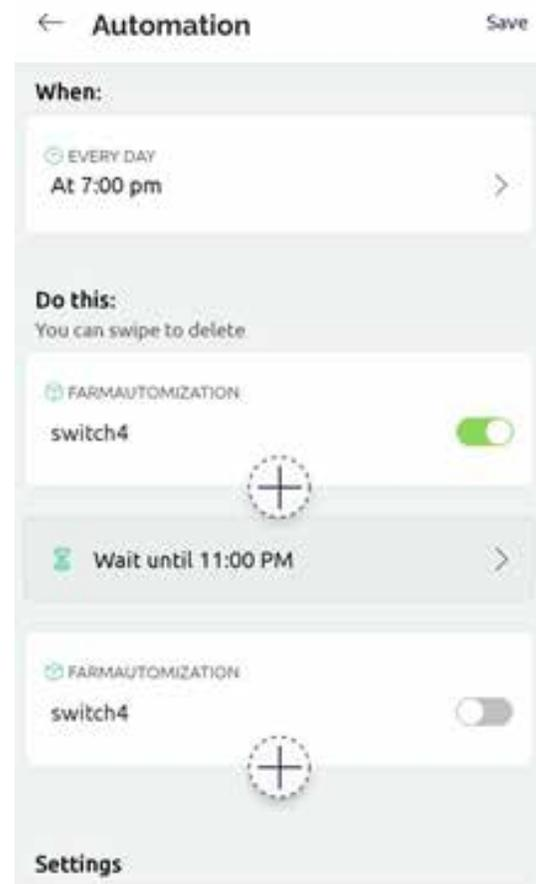
**Fig.8 Timer-based light on-and-off the system**
