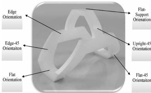
**Figure 2** Finger splint demonstrating six different build orientations
