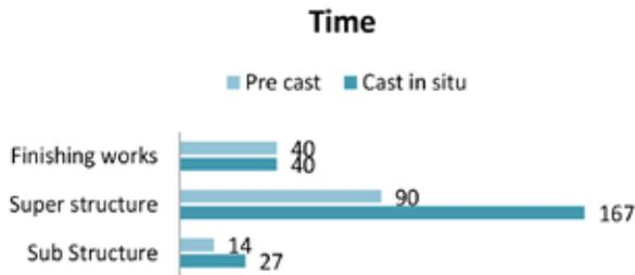
Fig 2. Time for Cast in situ construction and precast concrete construction.
