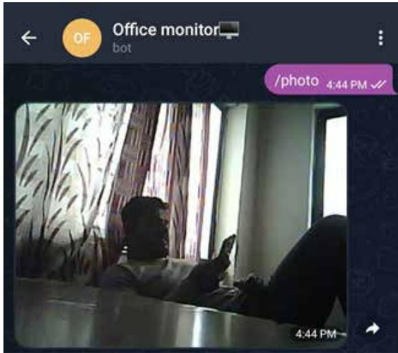
**Fig. 7 System responds to the “/photo” command from a user by capturing real-time photos**
