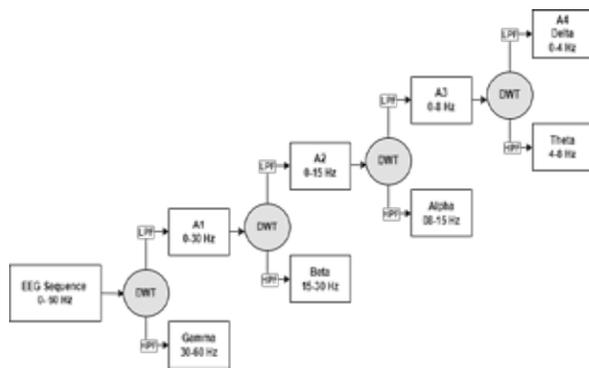
**Figure 3: Signal decomposition using Multi Resolution Analysis [2]**
