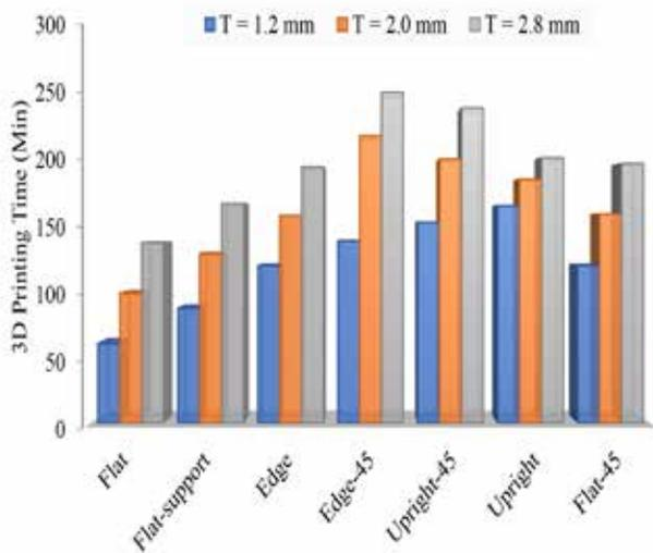
**Figure 4 3D printing time vs build orientation**
