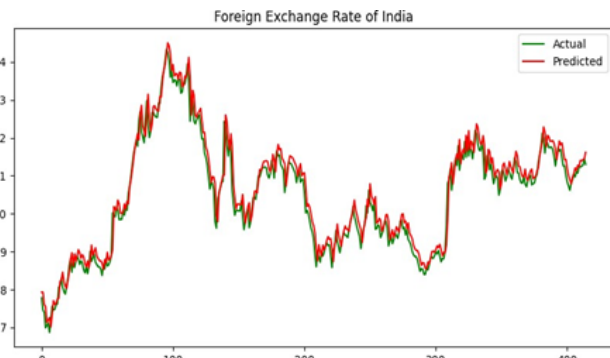
Figure 5. LSTM model Predicted and True rate values comparison.
