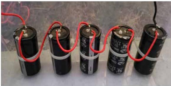
**Fig 4. Supercapacitor Bank**
