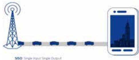
Figure-5: Single antenna transceiver system
