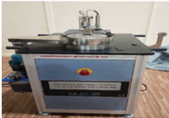
Fig 3. Pin on Disc Experimental Setup for Wear Testing
