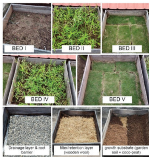
Fig. II Test Setup Showing Five Test Beds for Green Roofs and its Layers
