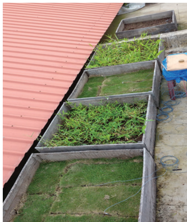
Fig. 1 Experimental Set Up Showing 5 Green Roof Test Beds (Bed No. I, II, III, IV & V – From Right To Left In The Image)
