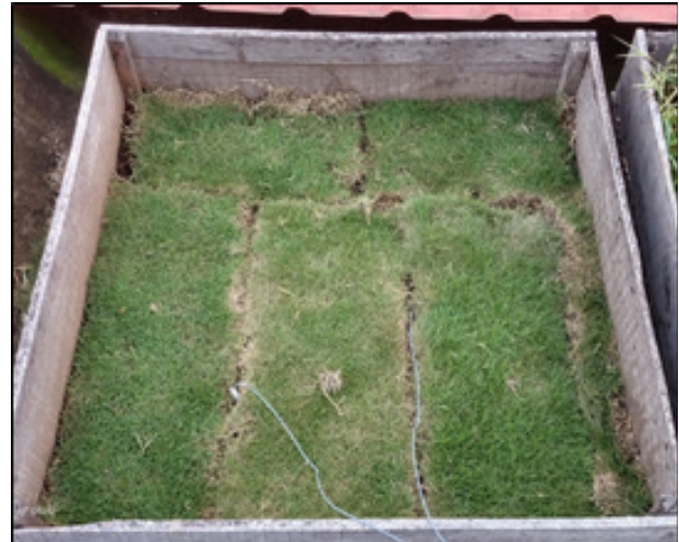
Fig. 3 Position of Temperature Sensors in One of the Test Beds (Test Bed No. 5, Garden Lawn and Garden Soil + Cocopeat Growth Substrate)
