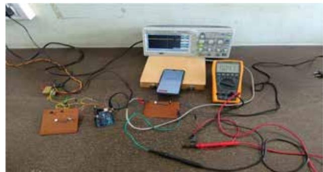
Fig 4: Hardware test of single phase automatic soft starter prototype
