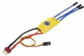
**Fig. 3. Electronic Speed Controller (ESC)**
