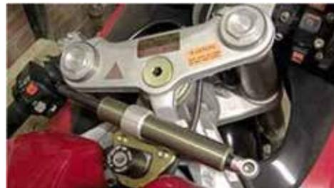
**Figure 3. Transverse linear motorcycle steering damper**
