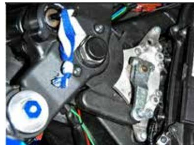
**Figure 4. Electronic steering damper with control arm attached to the upper triple clamp**
