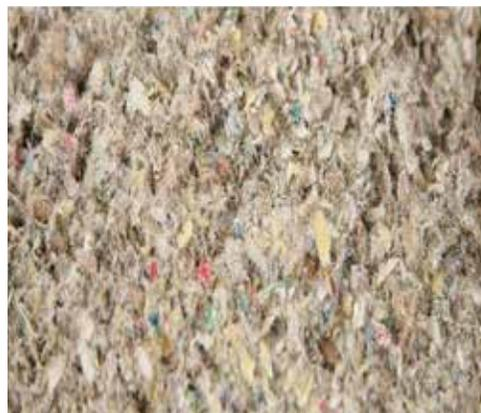
**Fig. 1 Raw form of Paper Cellulose (blown/sprayed)**
