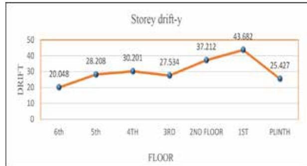
Figure 17: - Story Drift in Y direction for zone V
