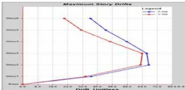
**Graph 5: For the load example, storey wander in the x and y directions: The two terms are Timex and Timey**
