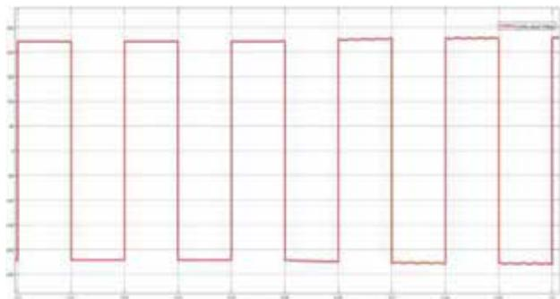
Fig.4.1.c– close loop output voltage waveform of inverter
