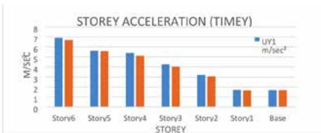
**Graph 3: Storey acceleration in the Y direction is compared for the load case TIMEY for models 1 and 2, respectively**
