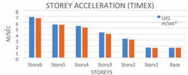
**Graph 2: Correlation of Storey accelerated for the load scenario in the x direction TIMEX for models 1 and 2 separately**
