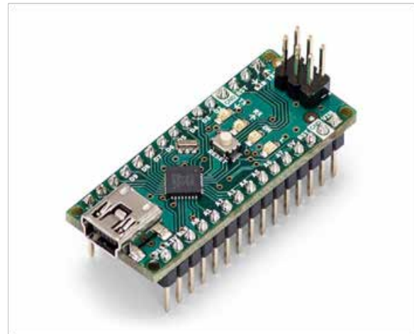
Fig. 6. Arduino Nano Board [2]
