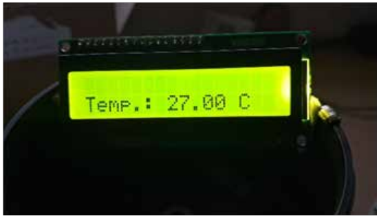
Fig. 8. LCD Display for displaying Temperature
