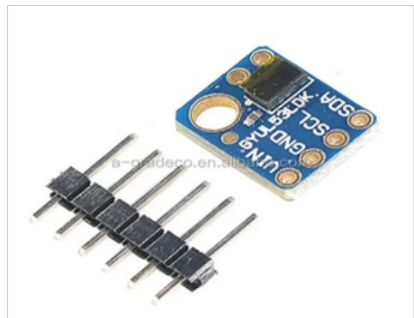
Fig. 7. Laser Sensor VL53L0X [3]
